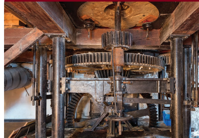
The hurst frame with main gearing and grinding stone (© Mike Bell)
