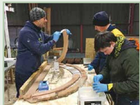
Boat building workshop - Constructing the strong-back and moulds.
